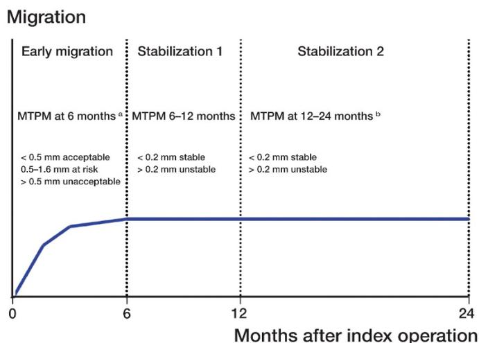
Figure 6 Thresholds of migration for knee replacements (Pijls et al., 2018)
