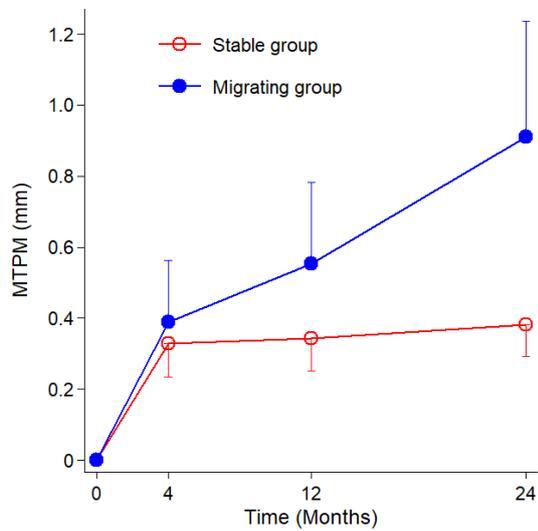
Figure 14 MTPM of the tibial component for the stable and continuously migration group (median and 95% CI). Adjusted from paper II.
