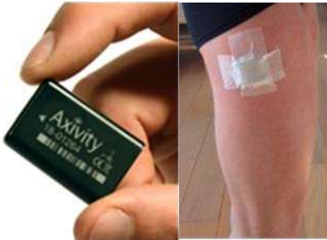
Figure 15 The 3D Axivity accelerometer used for monitoring patients' PA.
